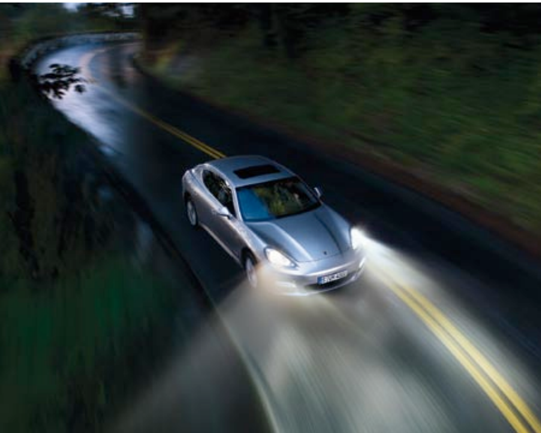
Cornering lights of the adaptive light system
